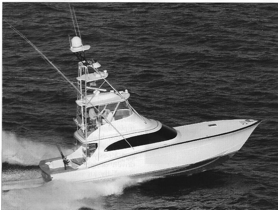
Jim Floyd and his crew at F&S Boatworks built this 50' (15.2m) convertible, a design developed with Matthews and Moesly. The boat is propelled by a pair of Volvo Penta IPS pod drives.
